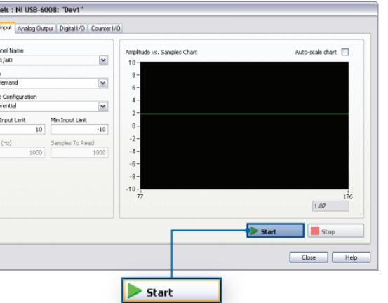
Take your first measurement in Measurement & Automation Explorer (MAX). Right-click the device and select **Test Panels**. After selecting measurement parameters, click **Start** to verify measurement functionality.
