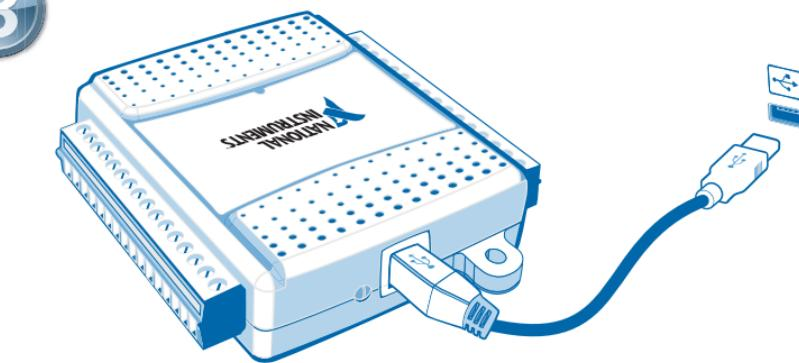
Connect shielded sensors and signals as described in the user guide. Then connect the device to a USB port on your computer.
